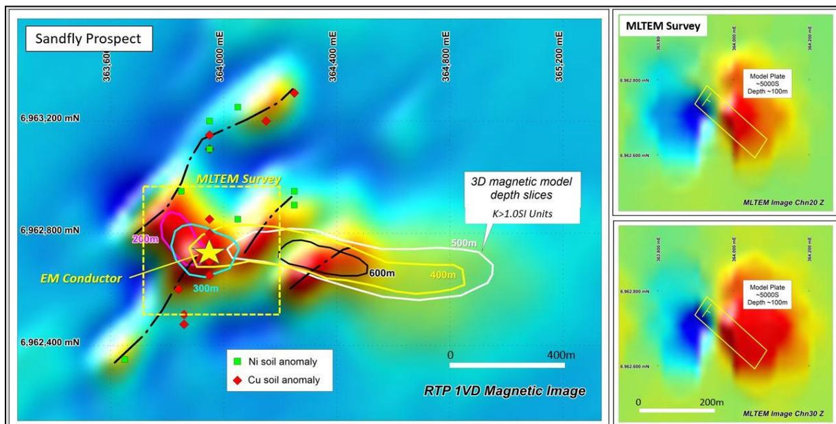
Figure 1: Sandfly prospect showing magnetic data plus EM anomaly/model (RHS) location.
