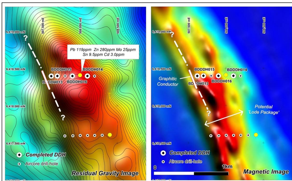
Figure 2: Tea Tree Prospect showing location of drill-holes on magnetic & gravity images
