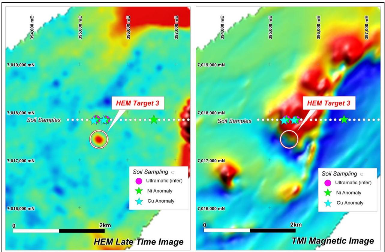
Figure 4: Morrisey HEM Target 3 showing association with magnetic target and soil geochemistry
