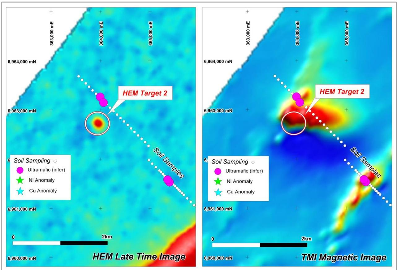
Figure 3: Morrisey HEM Target 2 showing association with magnetic target and soil geochemistry
