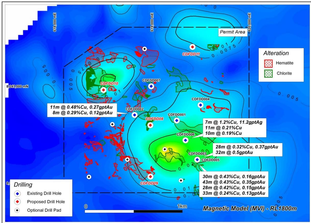
Figure 3: Cerro de Fierro magnetic model showing planned drill-holes and drill-pads
